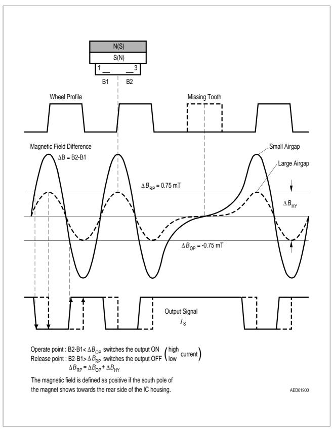
Figure 80 Sensor Signals Produced by a Toothed Gear Wheel, Example TLE 4923
