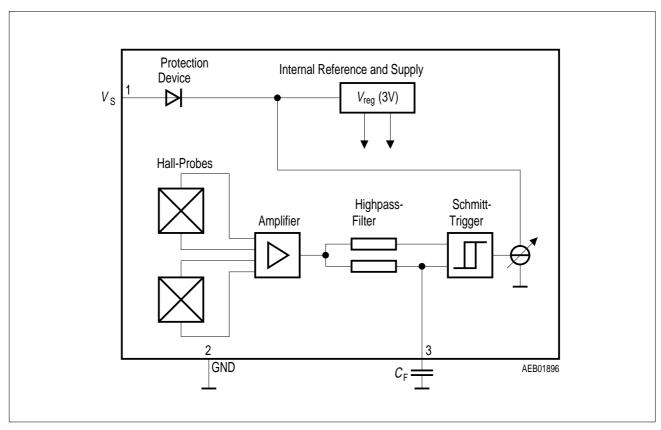
Figure 78 Block Diagram TLE 4923
