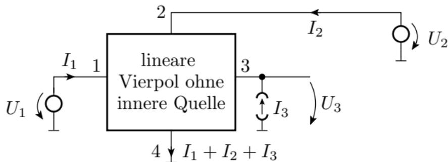
$$\begin{pmatrix} I_1 \\ I_2 \\ U_3 \end{pmatrix} = \begin{pmatrix} c_{11} & c_{12} & c_{13} \\ c_{21} & c_{22} & c_{23} \\ c_{31} & c_{32} & c_{33} \end{pmatrix} \cdot \begin{pmatrix} U_1 \\ U_2 \\ I_3 \end{pmatrix}$$
