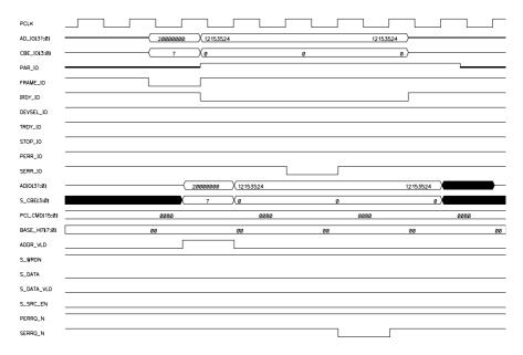
Figure 17-2 Target Write with Address Parity Error
