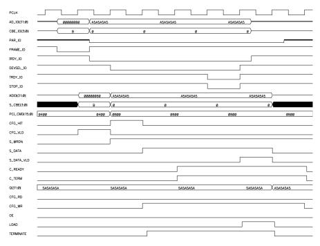
Figure 16-4 Configuration Write with Wait States
