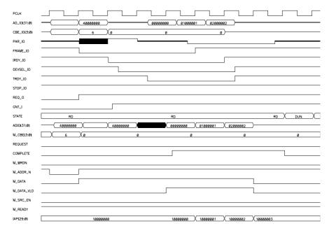
Figure 14-1 Initiator Burst Read Transaction
