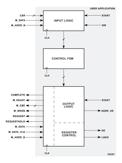
machine. This is represented in the block diagram of Figure 12-2, "Initiator Control Block Diagram".
