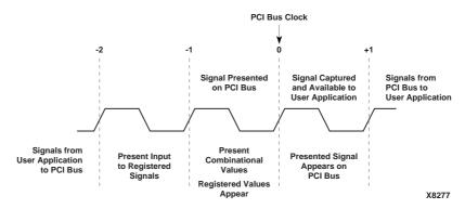
Figure 3-1 Signal Pipeline Delay
