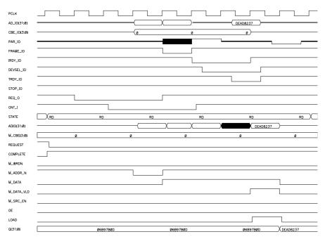
Figure 16-5 Initiator Issues Interrupt Acknowledge Cycle
