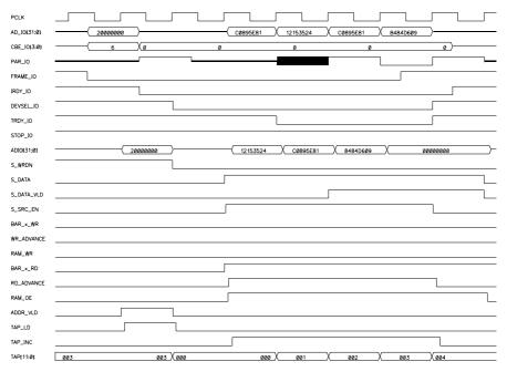
Figure 8-2 Target Burst Read Transaction
