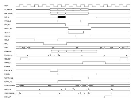
Figure 14-9 Burst Write with Target Disconnect
