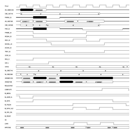
Figure 15-3 32-bit Target Responds to 64-bit Read
