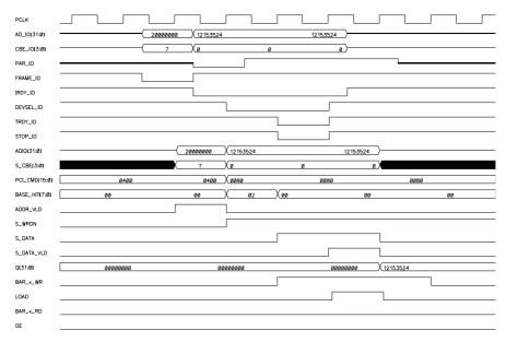
Figure 6-2 Target Write Transaction
