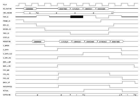
Figure 8-5 Burst Read of Target FIFO
