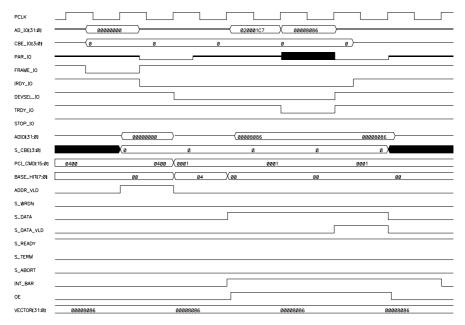
Figure 16-1 Target Accepts Interrupt Acknowledge Cycle
