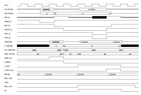
Figure 6-3 Target Read Transaction
