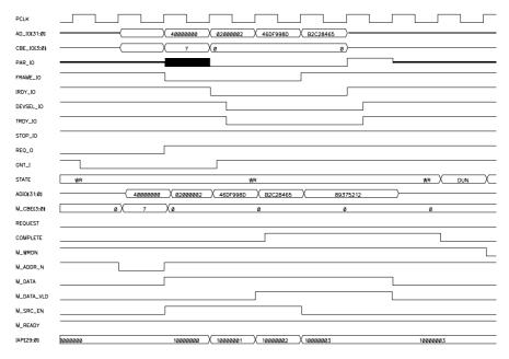
Figure 14-2 Initiator Burst Write Transaction
