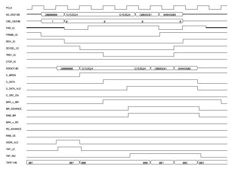
Figure 8-1 Target Burst Write Transaction
