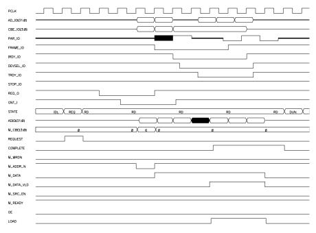
Figure 13-4 Three DWORD Initiator Read Transfer
