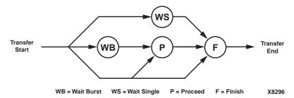
Figure 13-1 Permitted Data Phase Control Sequences
