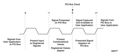
Figure 7-2 Control Signal Pipeline Delay
